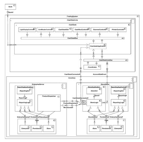
Figure 1 – SOFA architecture of the CoCoME assignment
