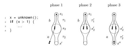
Figure 4. On-the-fly discovery of feasible covering paths
