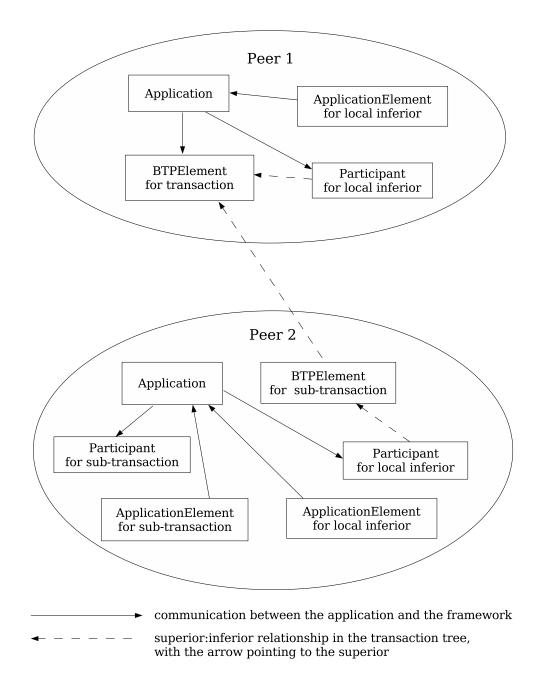
Figure 4.2: Structure of a Transaction Tree
