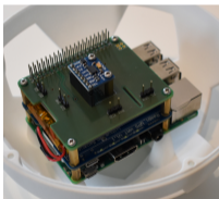
'Accelerometer': Receive data from sensor (ADXL345)
