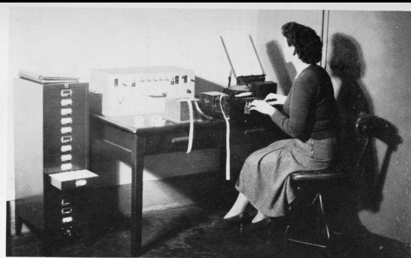
The library of tapes on which subroutines are punched is contained in the steel cabinet shown on the left. The operator is punching a program tape on keyboard perforator. By placing library tapes on the tapereader shown in the center of the photograph, the operator can copy them mechanically onto the tape she is preparing.
