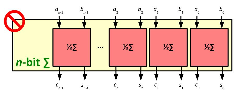
½-adder cannot propagate carry from previous additions (not enough inputs)
