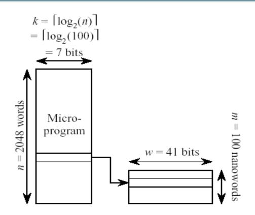
Microprogram Area =  $n \times k = 2048 \times 7$ = 14,336 bits Nanoprogram Area =  $m \times w = 100 \times 41$ = 4100 bits Total Area = 14,336 + 4100 = 18,436 bits
