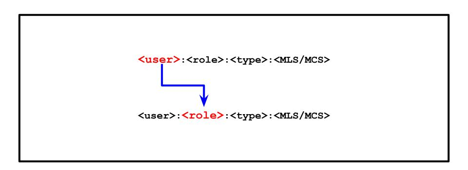
SELinux users can have multiple roles but only one can be active object\_r is a placeholder for Linux system resources system\_r is a placeholder for system processes
