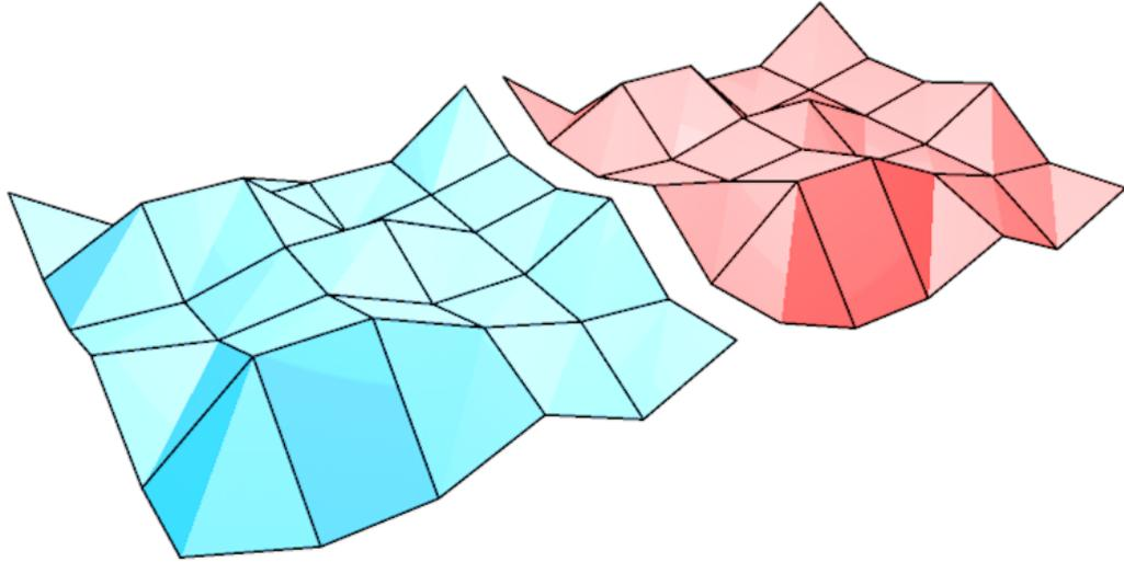
Figure 6.3: Illustration of the cracking problem in tessellation. Due to sampling the same heightmaps and using same tessellation factors for the adjacent edges, our tiles don't have this problem.
