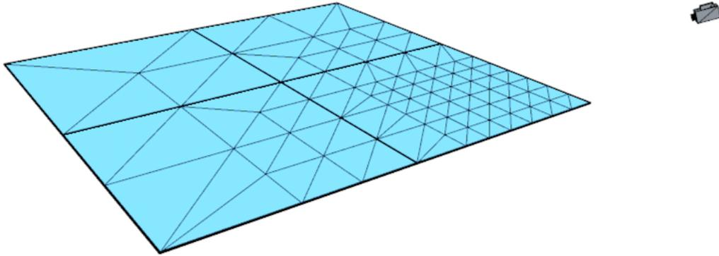
Figure 6.2: Illustration of the effect the view-dependent tessellation has on the tile vertex structure.
