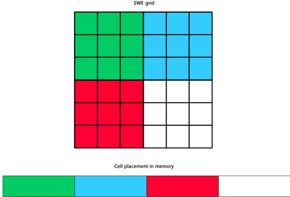
Figure 9.2: Proposed memory placement of cells in case of moving the SWE implementation to the GPU. Differently colored cell sets correspond to thread block sizes on the GPU, and are placed together in the global GPU memory array to better support coalesced loading.
