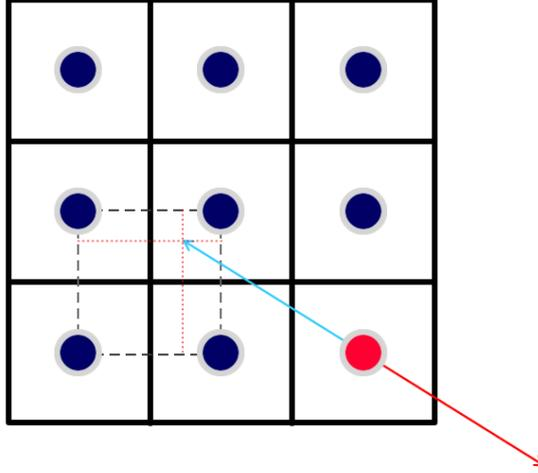
2. Using bilinear interpolation to find new velocity
