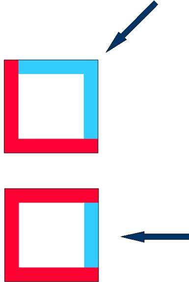
Figure 5.3: Visualization of how the wind direction impacts the creation of transitioning borders and damping zones of a tile. Blue borders represent Tessendorf-SWE transition, while red borders represent SWE-Tessendorf transition in the form of damping zones.
