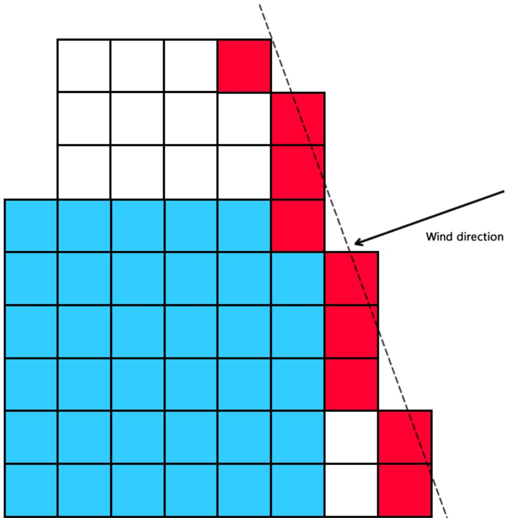
Figure 9.1: Example of irregular border shape used in place of the current square-shaped model corresponding to a tile. The original tile cells are blue, while the new cells are white and the fixed-height cells are red.
