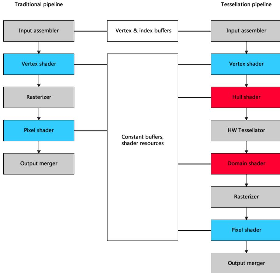
Figure 6.4: Comparison of the traditional graphics pipeline (left) and the tessellation-enabled pipeline (right). The arrows illustrate how the graphical data flow through the pipeline, while the lines represent the access to read-only data stored in buffers set by host code.
