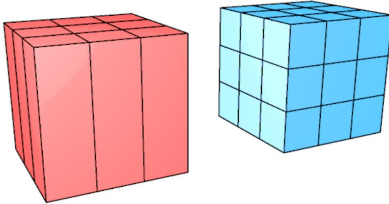
Figure 3.2: Visualization of the way the SWE (red) divide the simulation domain space compared to the NSE (blue).
