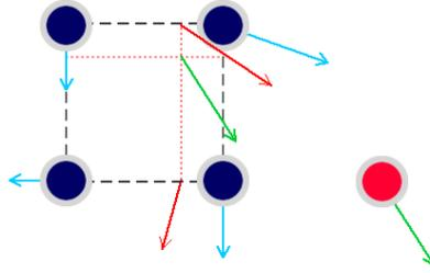
Figure 5.2: Illustration of Stam's advection scheme. In the first step, the current velocity of the particle (red) is inverted (blue) and used to find the approximate point of origin. In the second step, approximation of the point of origin velocity is found using bilinear interpolation based on the velocities of the surrounding grid elements (blue). The final interpolated velocity (green) is then assigned as the new velocity for the particle.
